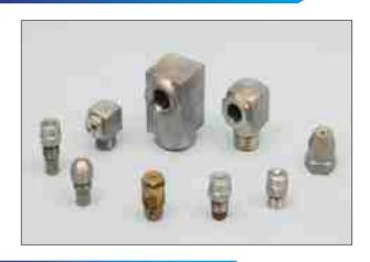
Hollow Cone Nozzles have an uniform liquid distribution. This uniform hollow cone atomization is possible due to Flow Geometry. Inside insert ensures efficient rotation of the liquids. Achieve narrow droplet size. The basic design of this nozzle is based on fundamental principle of axial swirling motion.
